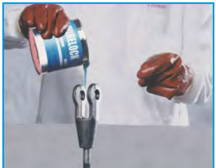
Upon mixing the compound should be poured immediately (Fig 7)
