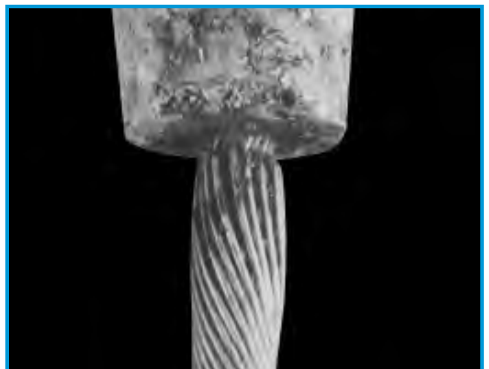
Typical example of the swelling of stainless steel rope due to crevice corrosion
